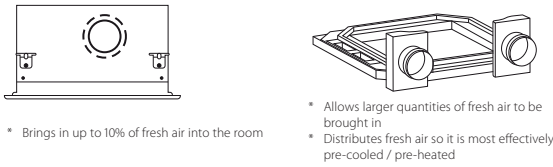
Fresh air intake opening in casing Optional fresh air intake kit
